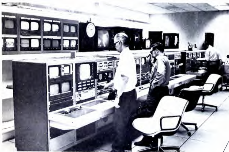
New master TV control has at its nerve center a video routing switcher to control all inputs and VTRs. Below is a view of a TV studio control room.
