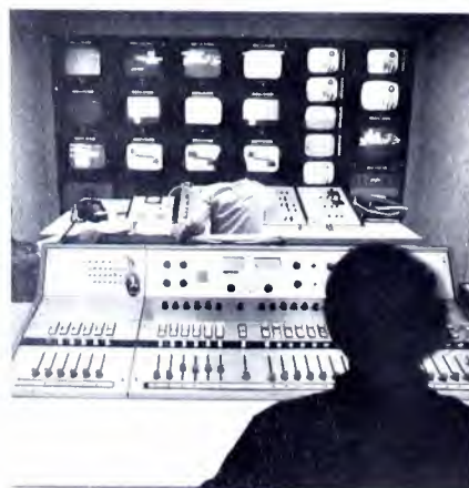
New master TV control has at its nerve center a video routing switcher to control all inputs and VTRs. Below is a view of a TV studio control room.
